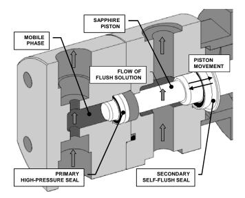
Figure 1-1. Self-Flushing Pump Head
